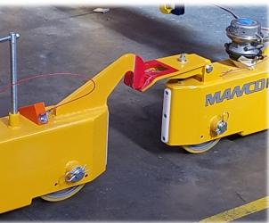
Manco Rail Rail-Track Trollies are designed to carry a pair of rail tracks up to 100m long in a train-like configuration
